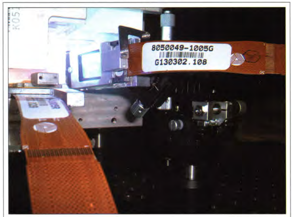
Fig. 3: Shown is an LCoS panel in a top-mounted configuration in a display system.
