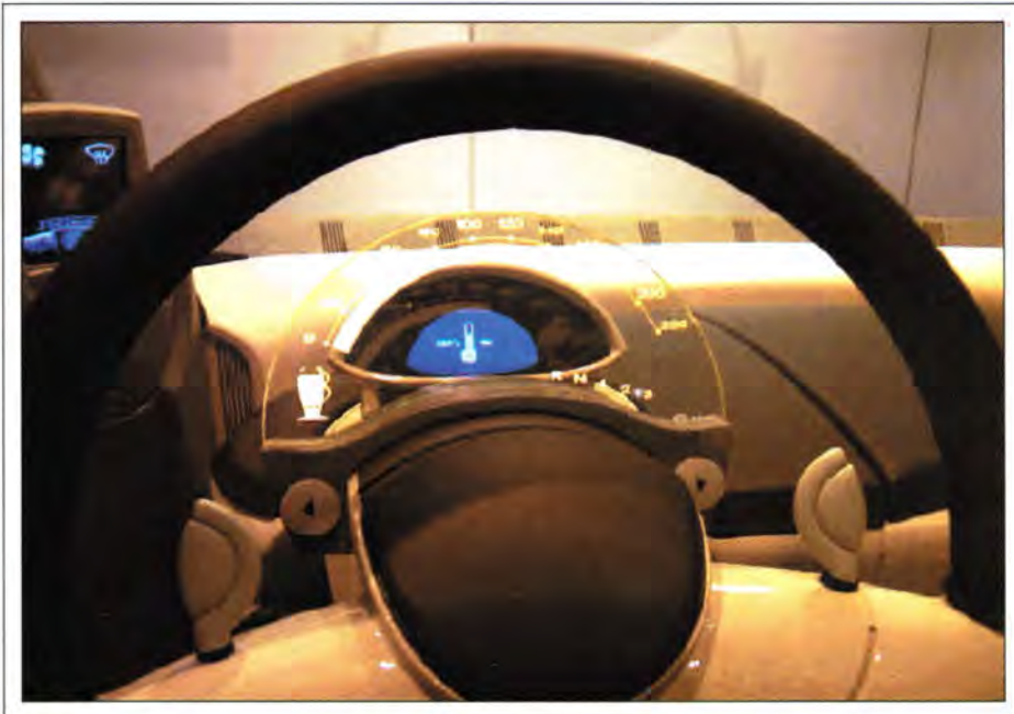
Fig. 6: The Johnson Controls–Planar steering-column display utilizes a futuristic transparent yellow EL device, with a blue alphanumeric gauge beneath it.
