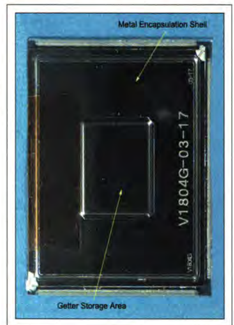
Fig. 1: This display module for an NEC cellular phone incorporates an OLED panel made by Samsung-NEC Mobile Display (SNMD). The display's glass substrate is epoxy-bonded to a flat metal can, which forms the back side of the display; the raised area in the middle houses the getter material.
