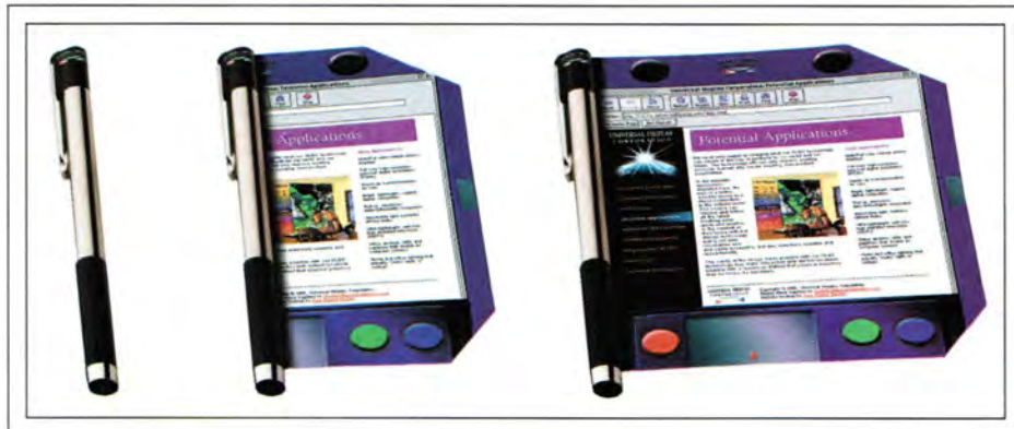
Fig. 3: A flexible AMOLED could enable a multipurpose communications device, such as this "pen communicator" concept from UDC.
