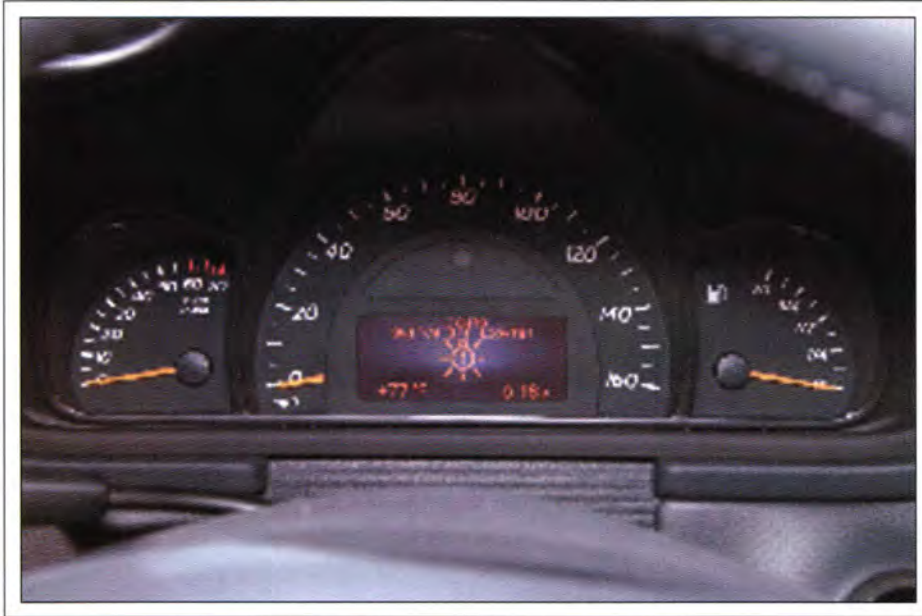
Fig. 2: The 2002 Mercedes 320 CS has mechanical analog gauges and a digital display which is a backlighted LCD.
